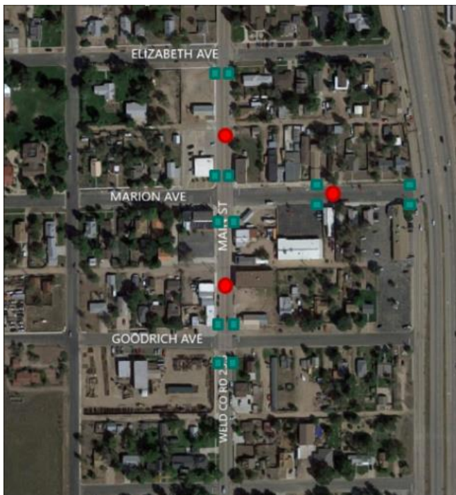
Figure 6.7: Possible locations of stormwater system access points (red) and inlet locations (dark green)
