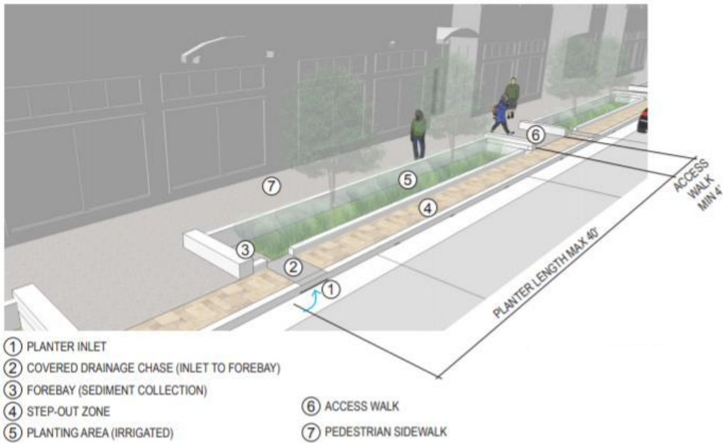
Figure 6.2: Isometric Diagram of stormwater planters (source: Ultra-Urban Green Infrastructure Guideline)
