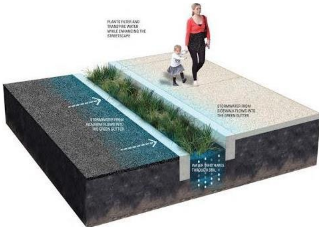
Figure 6.4: Stormwater planters, infiltration system. Image shows water traveling following the slopes of street and sidewalk.
